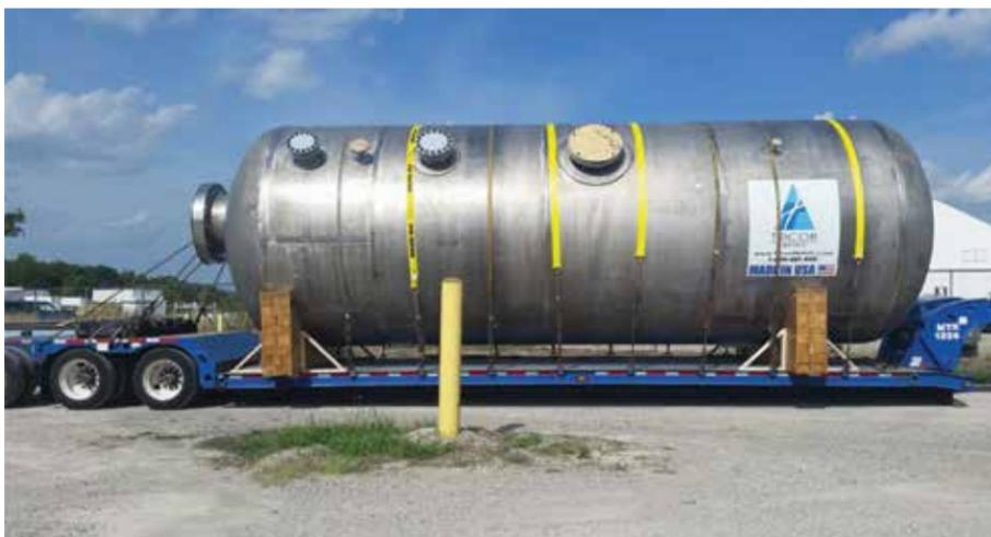
An American Society of Mechanical Engineers (ASME) Code tank, made from 0.875-inch thick titanium, grade 2.
