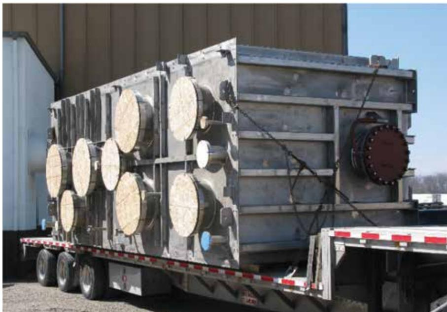
A titanium wastewater treatment tank.
